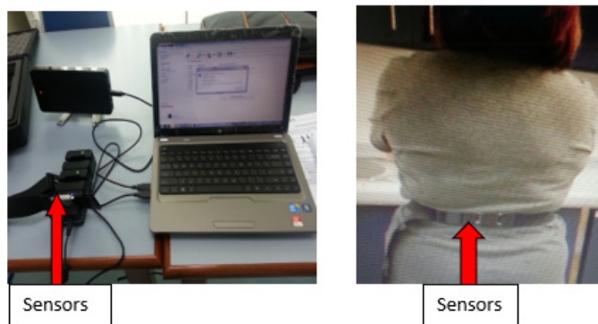
Figure 2 Kinematic sensors used and attachment of sensors at waist level
