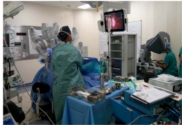
Figure 2: Difficult direct access to the patient once docking done and surgery started. Main surgeon operating using the Da Vinci TM surgical robot sitting away from surgical field
