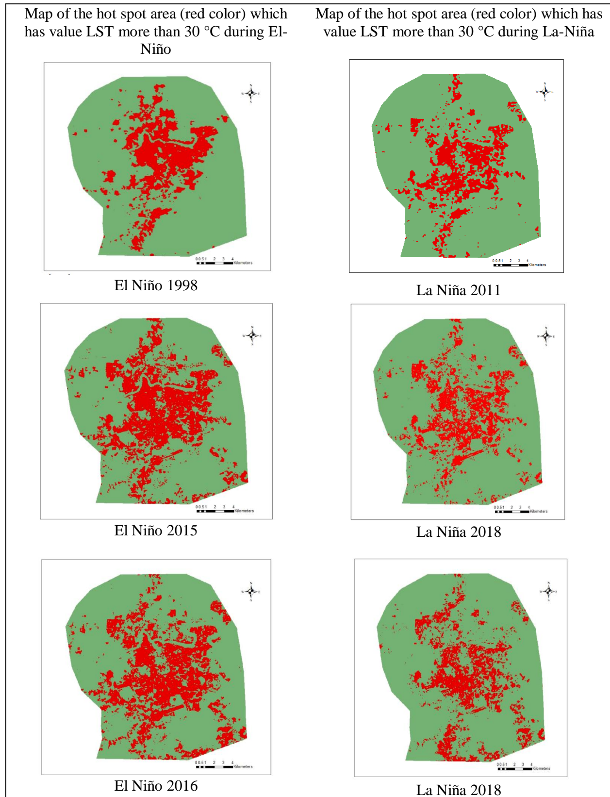
Figure 5: Spatial pattern of hot spot area that has a surface temperature of more than 30 °C (red color) during the occurrence of La Niña and El-Niño in Kuching City for Landsat satellites.
