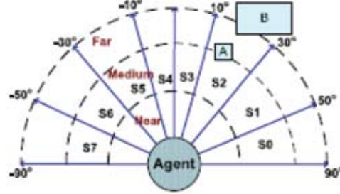
FIGURE 2. Example of Vision Field and Sensor's Region based on location
