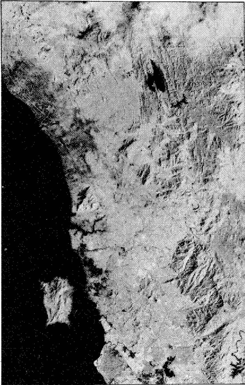
FIGURE 3: Landsat MSS imagery of north-west Peninsular Malaysia in band 7 (near infrared 0.8 - 1.0 \mu\text{m} ).
