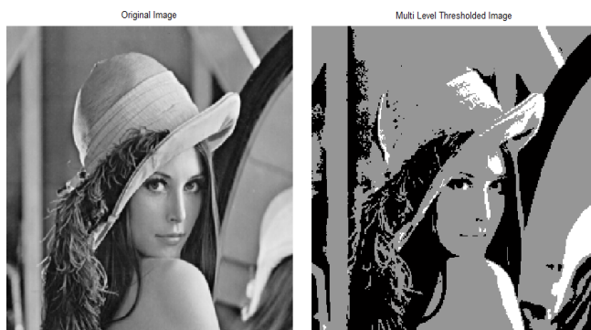
Figure 8: Output images and sample code for multiple thresholding based segmentation
